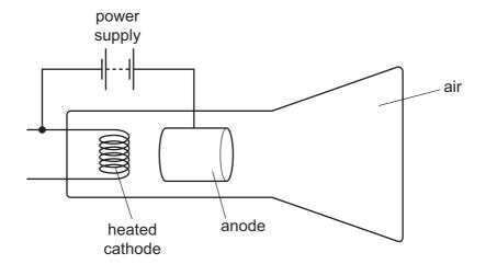
Which change should be made to make the tube work properly to produce cathode rays?
